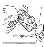
With your free hand, insert the Chuck into the Alignment Hole—make sure the flat spots on the Chuck match the flat spots in the hole.
