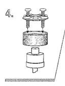
Remove worn wheel by twisting slightly and lifting wheel off shaft. Install new wheel and reinstall wheel retainer and screws. Don't over-tighten mounting screws Remove the wrench and replace the wheel access cover before turning on the machine
