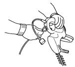
Position the loop over the cord retainer and pull back to secure.
